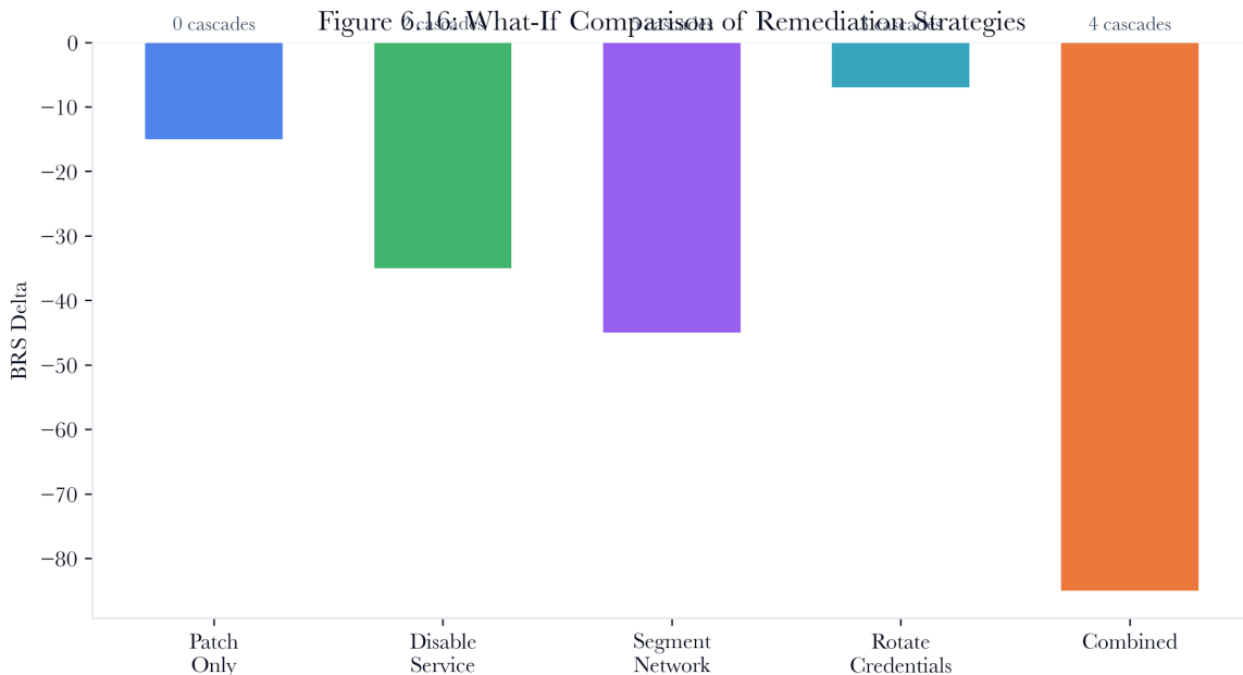
Figure 6.13: What-if remediation comparison. Patch, credential, segmentation, service-disability, and firewall actions can be compared based on predicted risk reduction and disruption before the production change.
